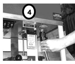
5. Plug the machine into a wall outlet. Keep in mind this unit should be on its own 20 amp circuit. We recommend that you do not use an extension cord; plug directly into the outlet. If you must use an extension cord, please make sure it is a heavy duty extension cord (at least 12 gauges).
