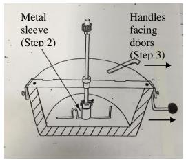
3. Make sure that the kettle arm and lid latch are facing the front of the machine. Place the kettle on its mounting bracket by slightly tilting it, sliding the small rods on the sides of the kettle into the slots on the bracket. Straighten the kettle until the gear, located on the top of the kettles drive shaft, is engaged with the motor drive.
