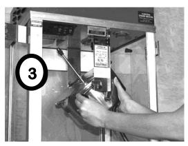
4. Insert the three prong kettle plug into the receptacle located on the inside of the machine on the underside of the ceiling of the unit, and twist gently clockwise to ensure a firm connection.
